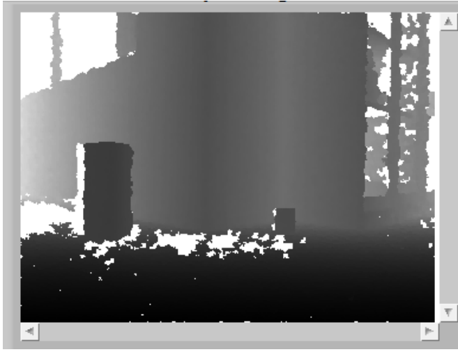
Fig. 5. Image obtained by converting the depth array to grayscale.
